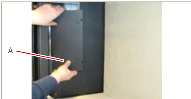
Fig. 24: Removing the revision cover
