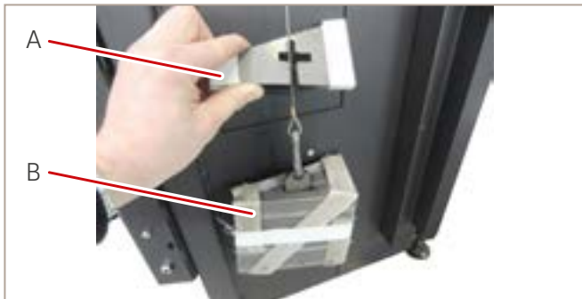
Fig. 19: Removing the balancing weights
