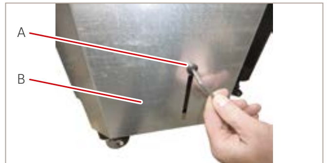
Fig. 17: Dismantling the transport restraints
