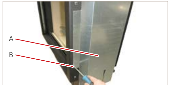
Fig. 16: Dismantling the weight shaft covers
