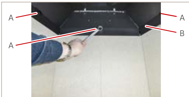
Loosening the fixing screws
