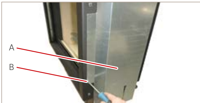
Fig. 19: Dismantling the weight shaft covers
