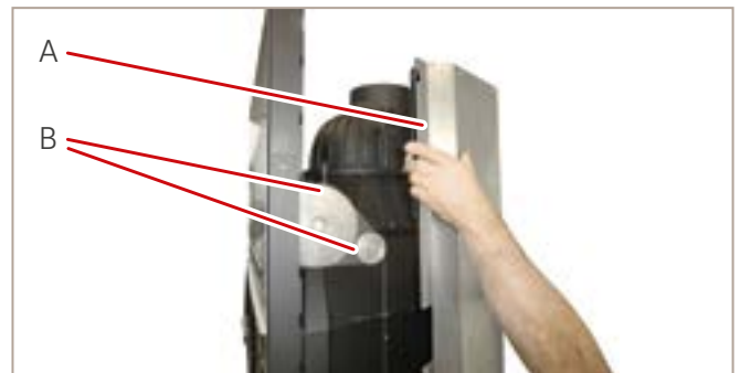
Fig. 21: Dismantling the weight shaft covers
