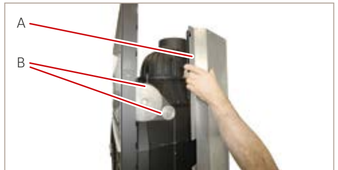
Fig. 17: Dismantling the weight shaft covers
