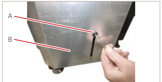
Fig. 16: Dismantling the transport restraints
