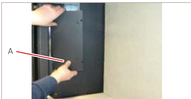
Fig. 23: Removing the revision cover
