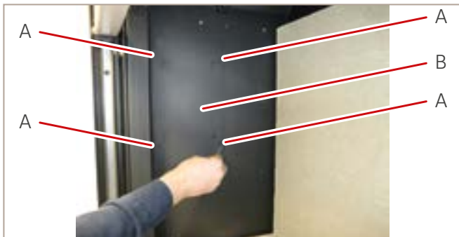
Fig. 22: Dismantling the revision cover
