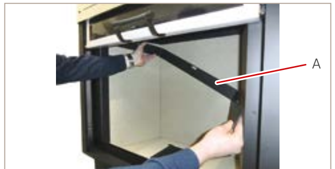
Fig. 21: Removing the fire box inner lining
